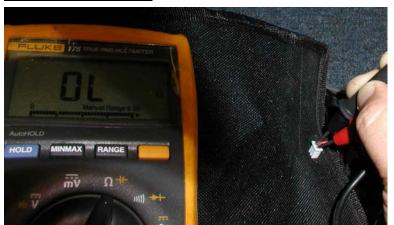
Place the probes on the connector as shown and turn the volt-meter to read  $\Omega$ , the reading should be OL (open circuit). Once the brake lever is depressed, the reading should be  $\sim 0.5~\Omega$ ; otherwise, the brake cable is bad.
